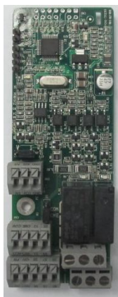
IO extension card EC-IO501-00
